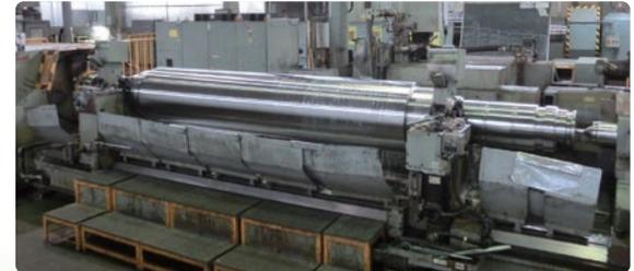
Low Frequency Progressive Induction Hardening + Sub-zero Treatment + Tempering
