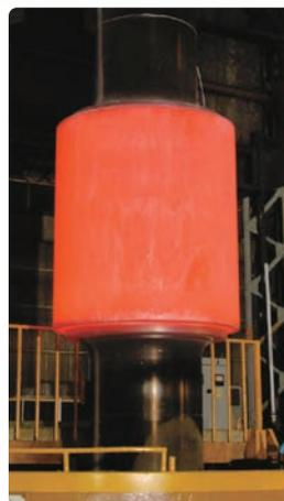
11 Low Frequency Static Induction Heating Equipment
