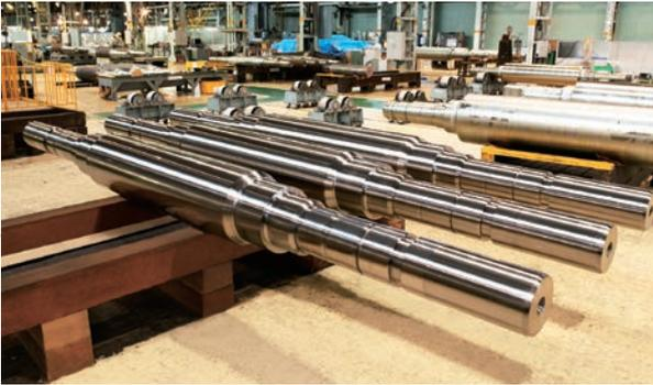
Work Rolls for Electric Steel Sheet Rolling Mill
