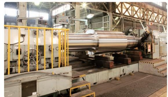
14 CNC Large Scale Finishing Lathe
