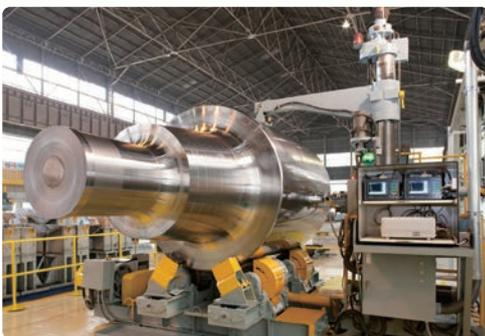
9 Large-size Automatic Ultrasonic Flow Detection Machine
