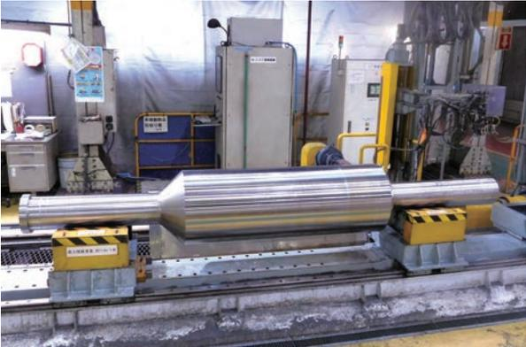
Middle-size Automatic Ultrasonic Flaw Detection Machine
