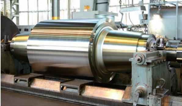
Back Up Rolls for Hot Strip Mill
